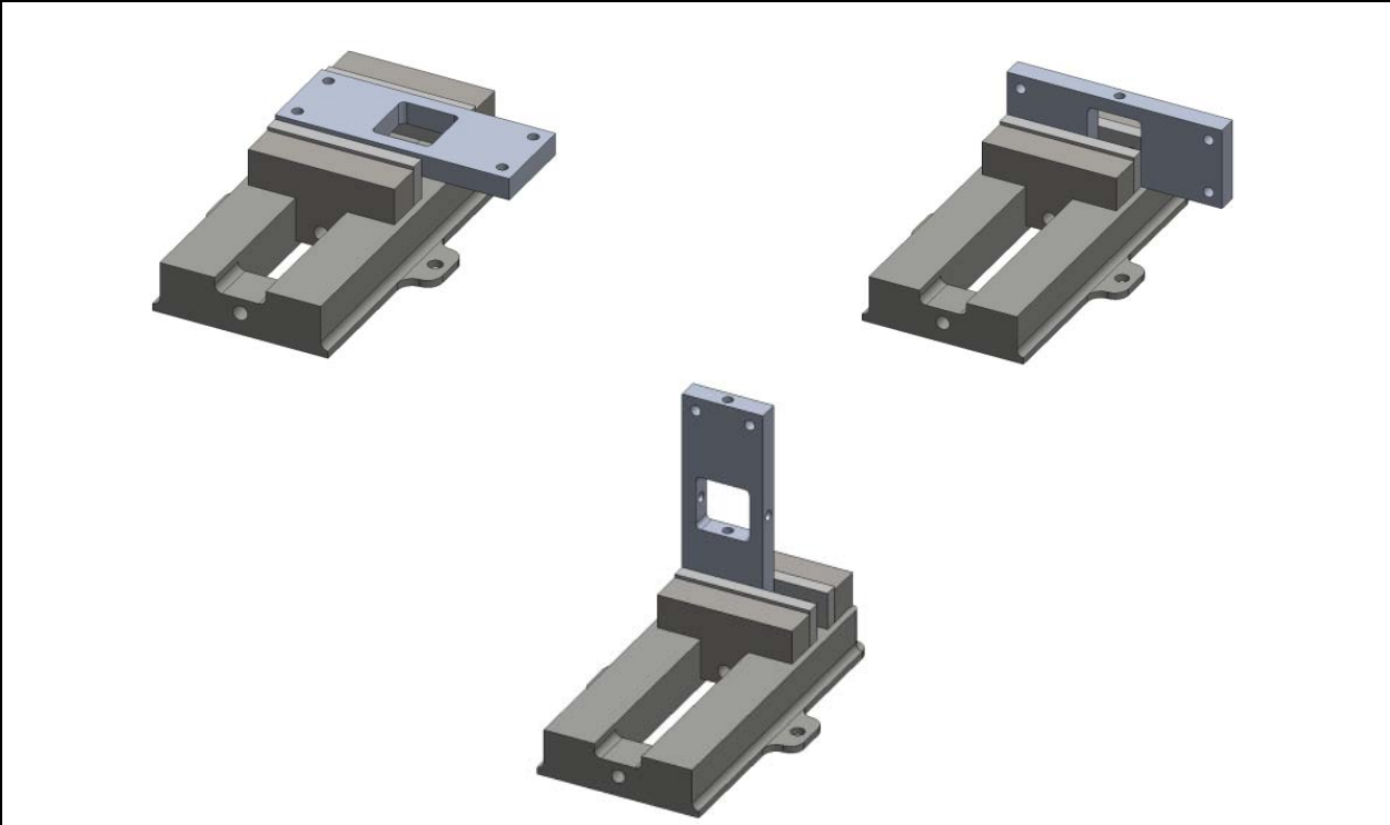
Figure 3.1 – Multiple setups required for a part that cannot be machined TOP DOWN
