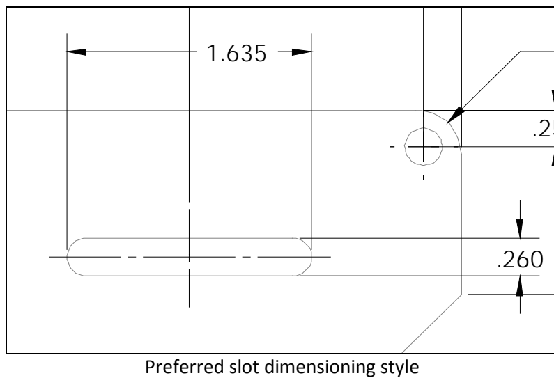
Figure 10.4 – Dimensioning of a slot length
